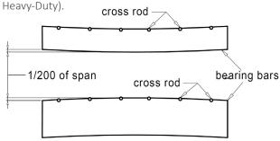
**Transverse Bow.** Before banding, the transverse bow should be less than 1/8" per foot of width.
