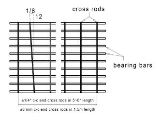
**Cross rod Position.** The top of cross rod should not project more than 1/16" above the top of the bearing bars for standard grating (1/8" for heavy duty) and should not extend more than 1/8" from side of bearing bars.
